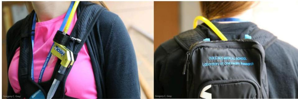
**Figure 1.** Aerosol sampler attached to a personal backpack carrying an SKC Airchek pump worn by researchers.
